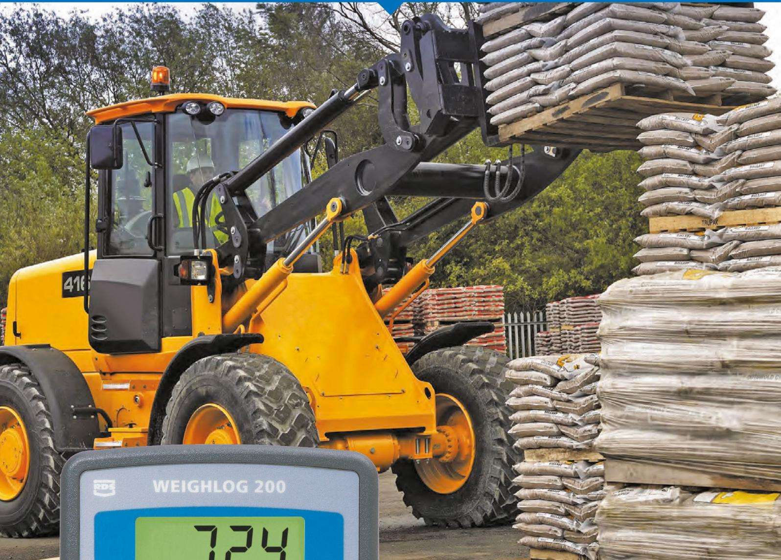
**A user friendly onboard weighing system for vehicles with or without cabs**
