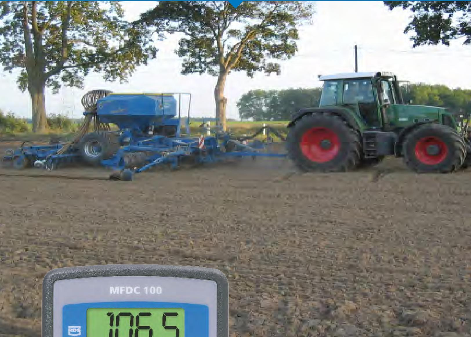
**A range of control systems to monitor the operation and control the tram lining of conventional and pneumatic seed drills**
