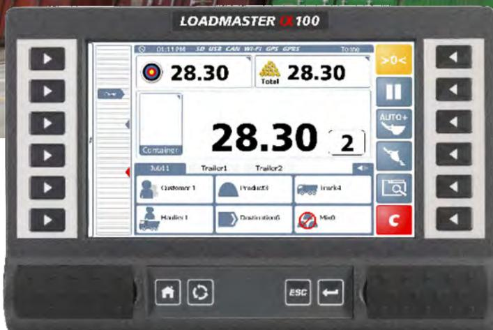
**A dynamic on-board weighing system specifically designed for reach stackers and meeting SOLAS 2016 requirements**
